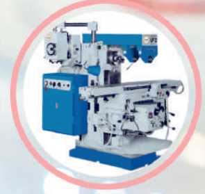
MODEL: BHARAT FRITZ WERNER - UF 3.5 (UNIVERSAL MILLING MACHINE)
